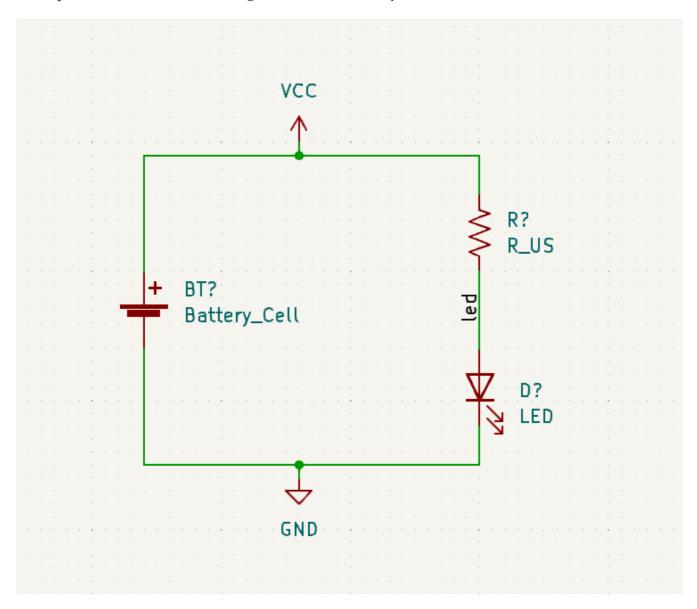
Note that labels and power ports with the same name are connected together. Another GND power port or wire labeled led on this schematic page would be shorted to the existing one, even without wires visually connecting them.
